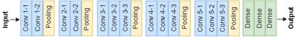
Figure 5. VGG16 with 13 Convolutional Layers and 3 Fully Connected Layers [8].
