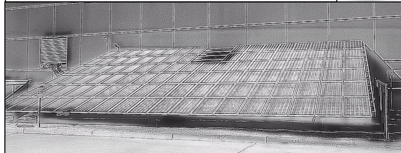
Thermal/infrared camera can capture PV semiconductor defects and faults not visible to the human eye.
