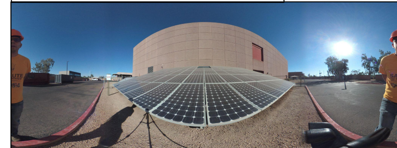
360-camera useful for collecting wide field of view at low hardware cost. 3D-model of physical environment can estimate geometric shading pattern.
