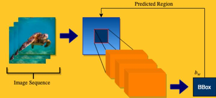
Fig. 3: Model of object detection + bbox retrieval
