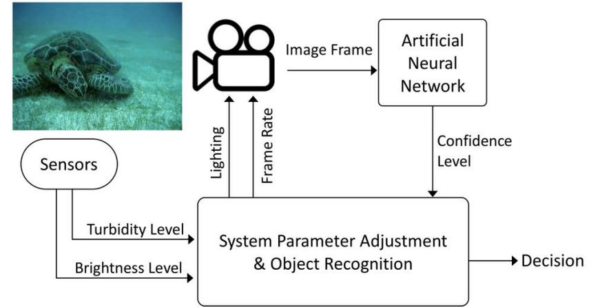
Fig. 1: Block diagram of the recognition system
