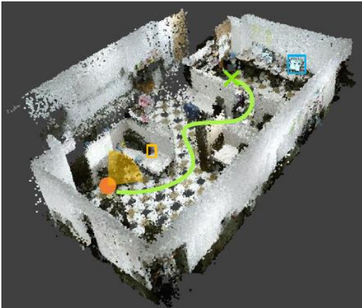
Figure 2. A 3D reconstruction of the room is generated from 2D camera imagery [8].
