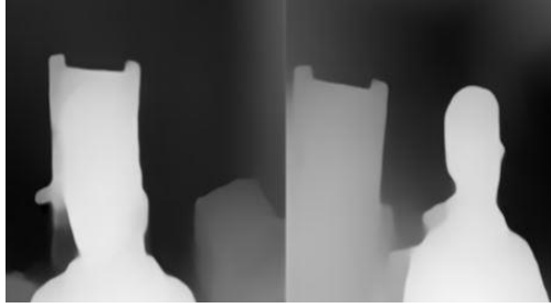
Figure 5. Midas depth estimator depth map output generated by RGB input data from multiple cameras
