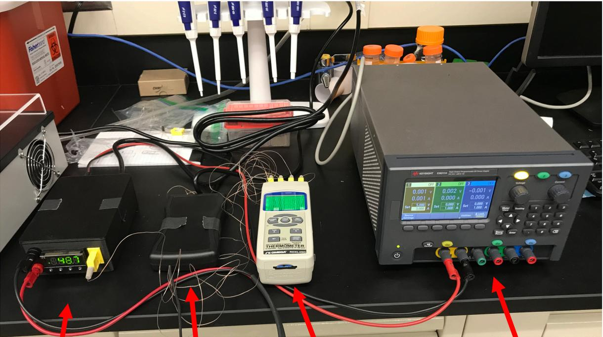
PID Controller    Reader    Thermometer    Voltage Source
