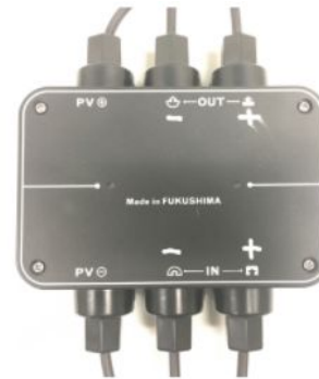
Smart Monitoring Device (SMD) [1] Helps diagnose solar faults
