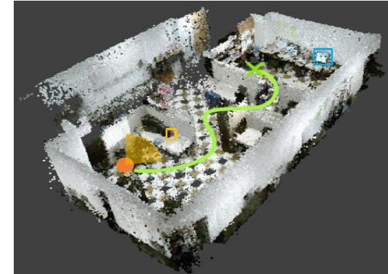
Figure 3. 3D Room Mapping SLAM Algorithm Output
