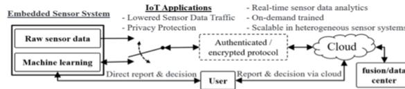
Fig. 2. Embedded sensor and machine learning platforms.
