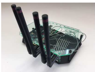
Fig. 4. The LimeSDR RF 2x2 MIMO transmitter and receiver [21].
