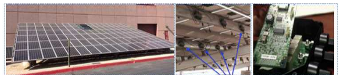
Fig. 1. a) ASU Solar Monitoring facility [10]; b) the SMDs attached to panels; c) SMD electronics, relays and radio.
