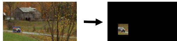
Fig.4. Example of bounding box being used to subsample an image. [2]
