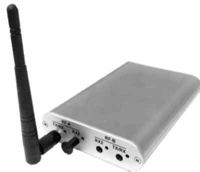
Figure 3. The USRP B200 Radio, with only one antenna attached at the Tx port.
