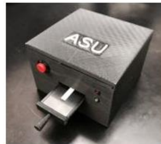
Figure 3. PoC HPV testing box that will be placed inside of the climate chamber for detection process.
