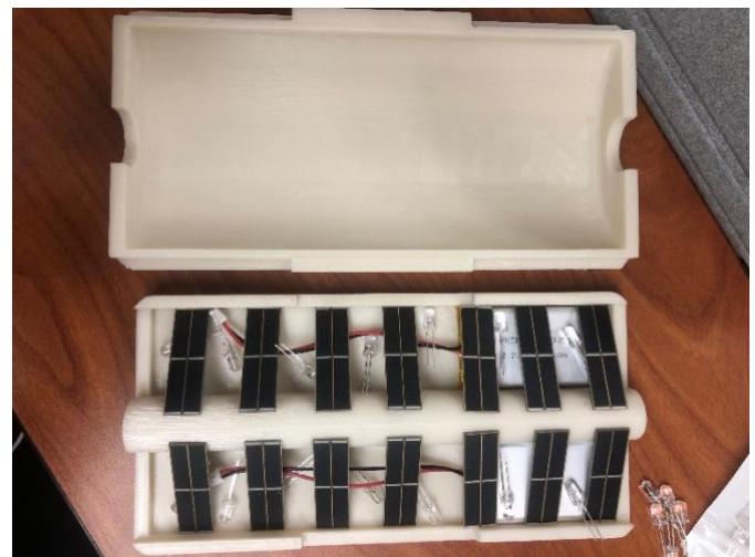
Figure 22: Initial prototype printed from ABS with solar panels, lithium polymer batteries, and LED lights
