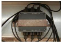
Figure 1: An SMD device setup to its corresponding solar panel.
