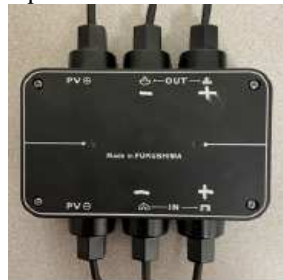
Figure 1 The smart monitoring device (SMD) for solar panel monitoring and control.
