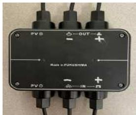
Fig. 1 The smart monitoring device (SMD) for solar panel monitoring and control.
