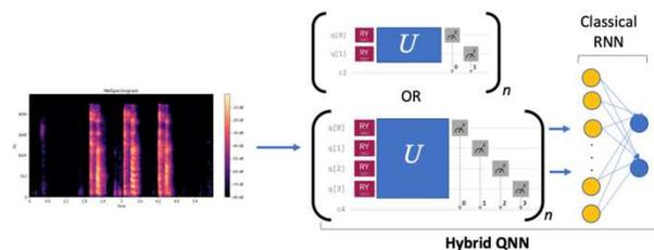
Fig. 3. A basic framework for the quantum ML data pipeline used in this study. Quantum convolution is performed in order to extract features from log-mel spectrograms and the features are then used to train a classical recurrent neural network.
