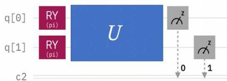
Fig. 1. A block diagram representation of the two-qubit circuit used for audio feature extraction.
