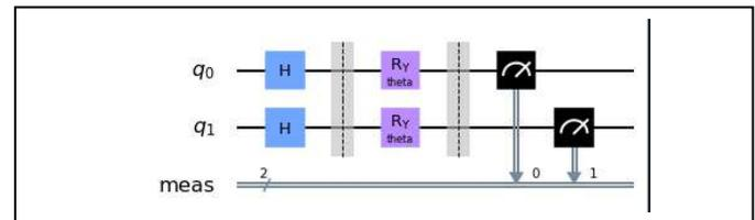
Fig. 5. The quantum circuit using Qiskit [77].
