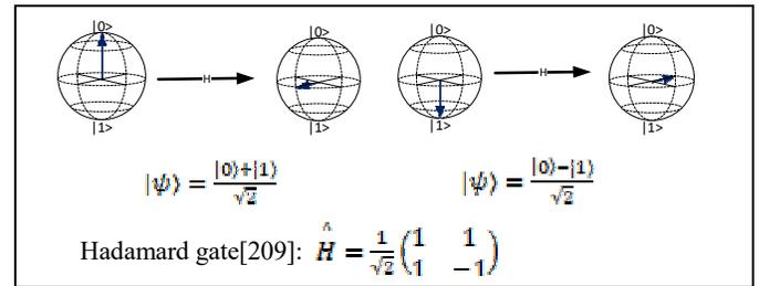
Fig. 4. The application of a Hadamard matrix to a qubit is shown in terms of a Bloch sphere.
