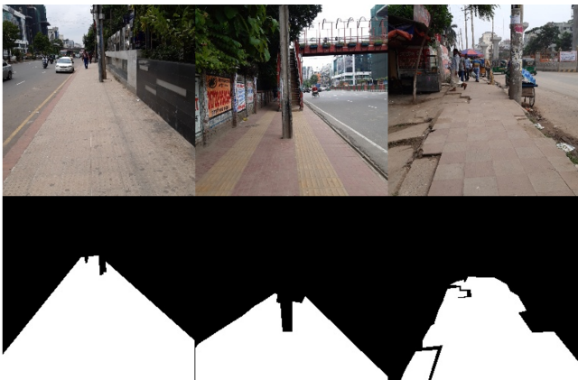
Figure 3: Example pictures of Bangladesh footpaths and corresponding masks to the footpaths dataset Source: [13]
