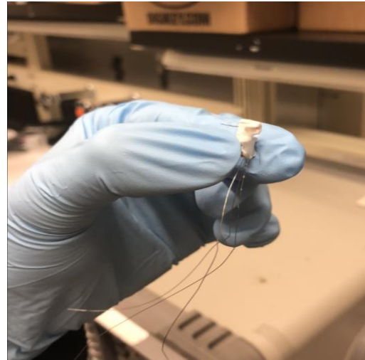
Fig: Disassembled FreeStyle sensor
