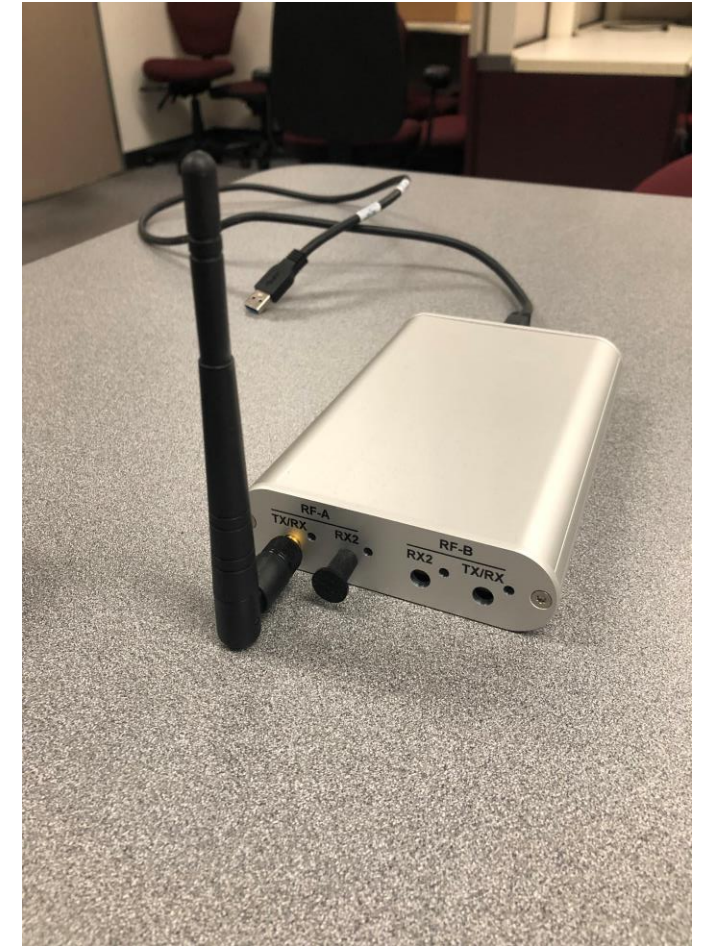
Figure 2: The USRP B200 Radio with an antenna attached at the Tx/Rx port.
