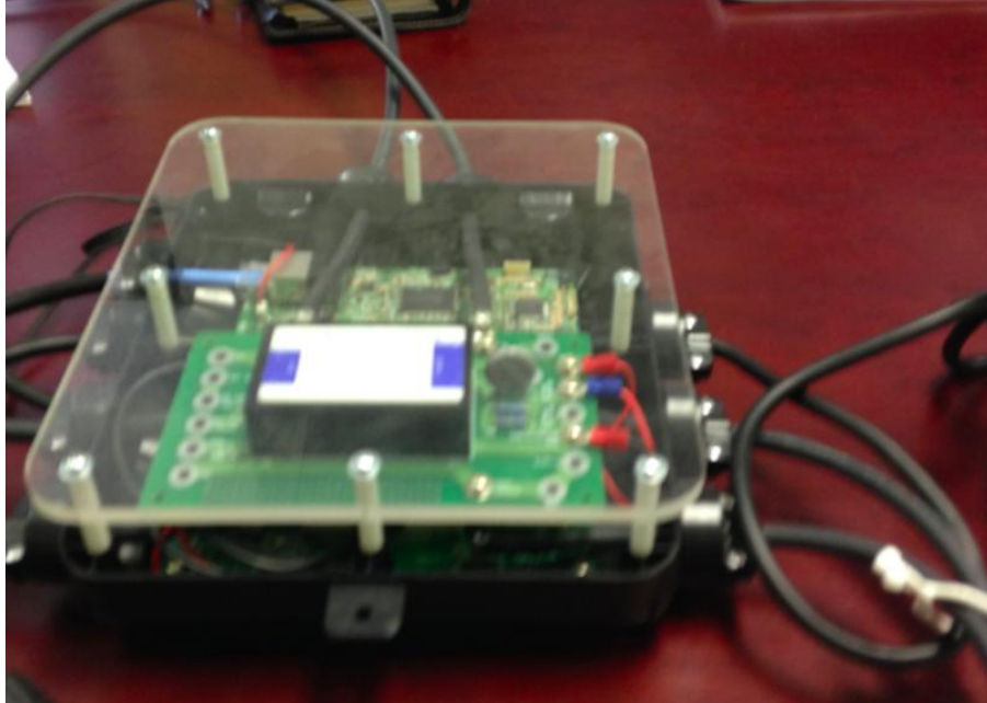
Fig. 3. Prototype sensors and communications hardware for intelligent Networked Array Monitoring. These sensors monitor irradiance, temperature, voltage, current and have hardware to enable local and cloud computing and communications capabilities.
